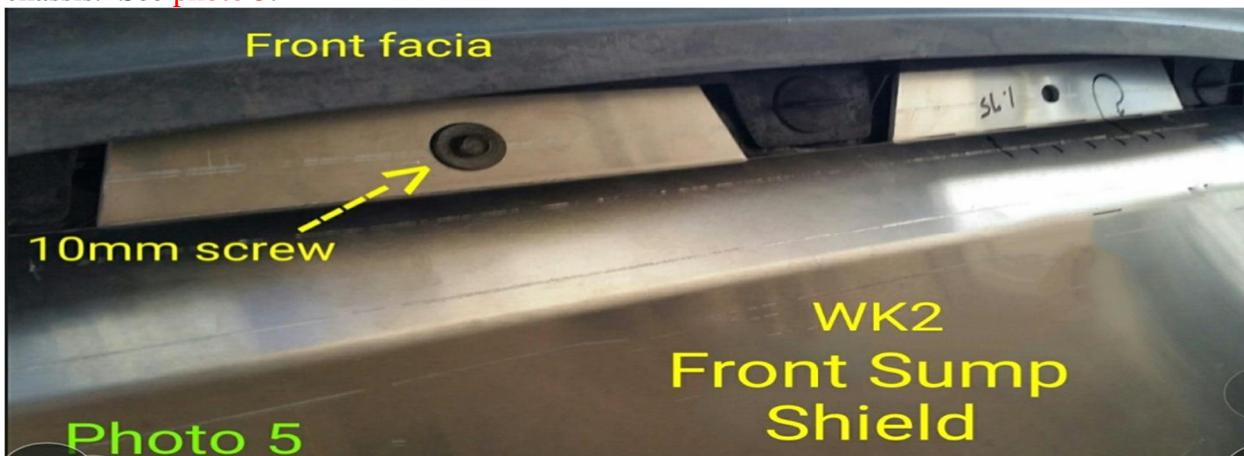
Locate the three 10mm screws and add some blue Loctite to the threads. Now place them through the shield holes and partially screwing them back into their A, B and C locations.
